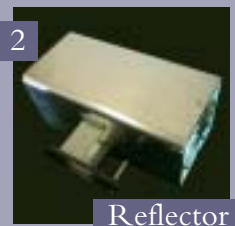
2 Reflector The aluminum Reflector Tube increases the intensity of the UV Lamp. Installed parallel to the air flow, it increases exposure of contaminants to UV rays.
